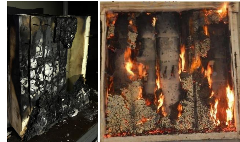
Figure 04: The samples after the tests VHFlux and AS 1530.4
